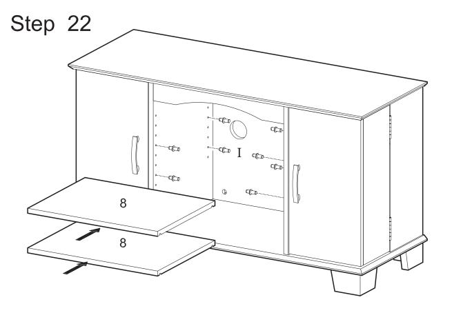
Insert shelf support pins (I) into the stand assembly at desired shelf heights. Carefully slide shelves (8) into place resting on shelf support pins (I).
